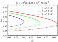
The dependence of the resonant positron energy (in units of the total energy of the initial gamma-quanta) on its outgoing angle for a different number of absorbed wave photons for two laser intensities. Solid lines correspond to the solution with the "plus" sign, dotted lines – with the "minus" sign. The initial parameters are equal to:
