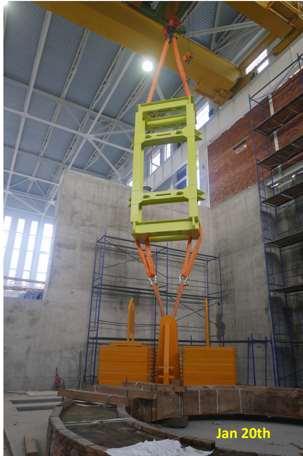
MPD Hall crane weight test
