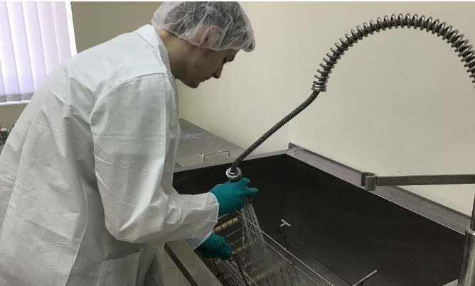
Glass cleaning with ultrasonic wave & deionized water
