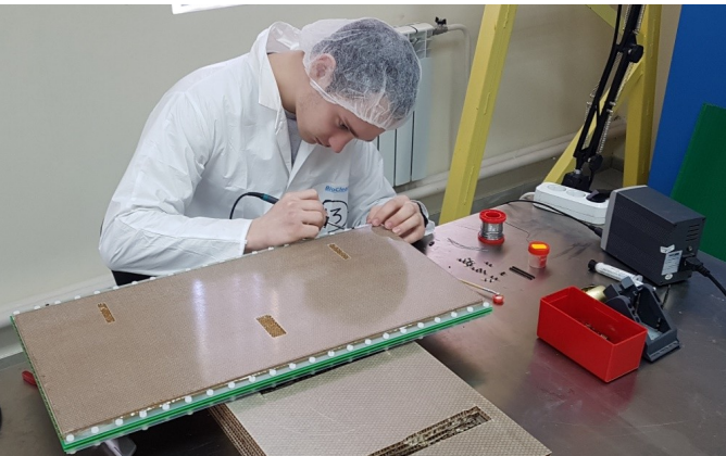
Soldering HV connector and readout pins
