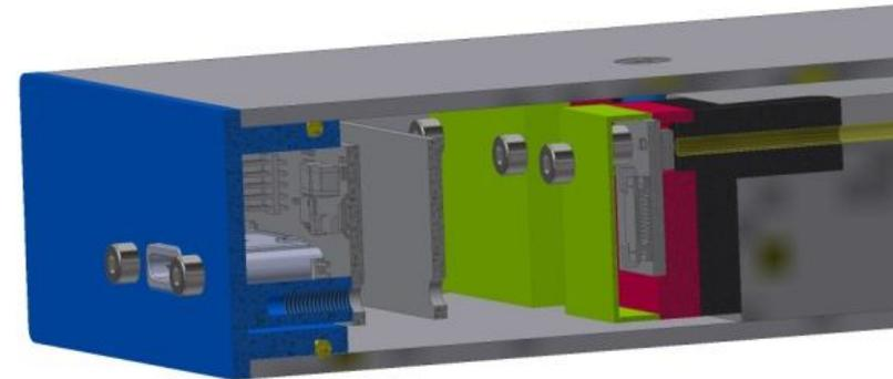
View of the area between the end of scintillator and End-Cap
