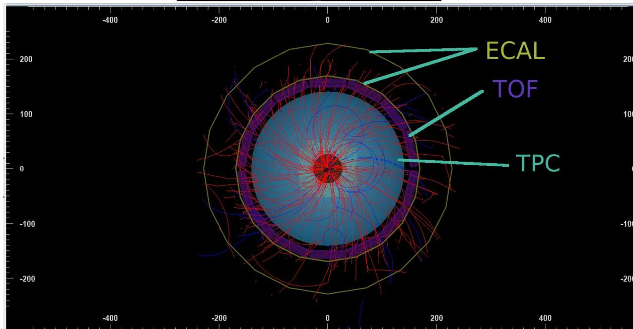
Visualization of central gold-gold collision. Positive pions are marked as red, whereas positive muons are blue. It can be seen that a lot of pions vanish in ECAL without production of muon
