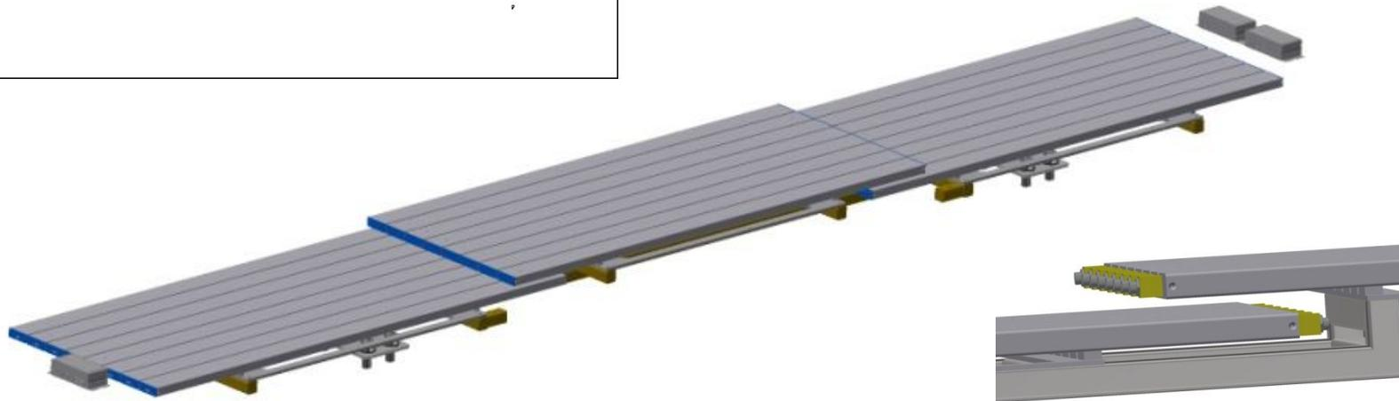
MCORD module consist three sections and installation frame.
