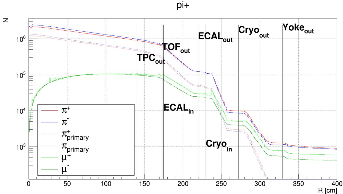
The plot was made by calculation of the total number of particles at  $|Z| < 190$  cm and  $p > 1$  MeV/c as a function of distance from axis beam, simulation was done for 19k Au-Au central collisions (centrality 0-5%) at 11 GeV. The primary particles does not include the particles from strong decays.
