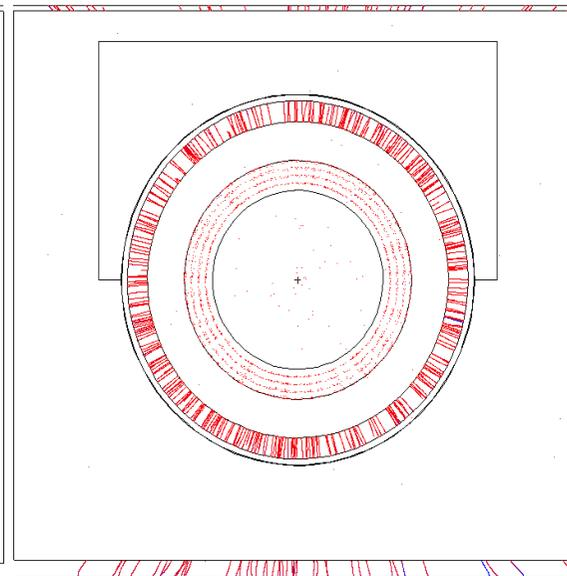
MCNPX calculated central muon transmission through the MPD, MCORD and concrete walls.
