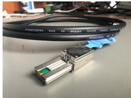
2xSAS-external cable + 1xEthernet cable for one section (8 scintillators)
