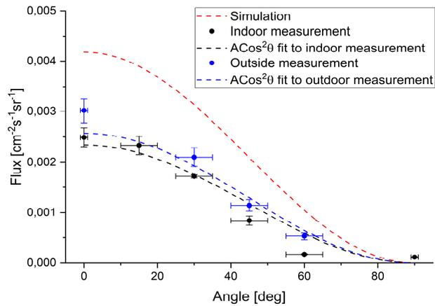
The Cosmic Watch detectors measurement results at Dubna (July 2019y). Flux dependence on the direction with respect to the azimuth (coincident mode).
