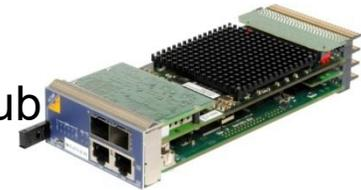
**For several MTCA's one main MCH concentrates data from slave MCH's to generate the final muon trigger**
