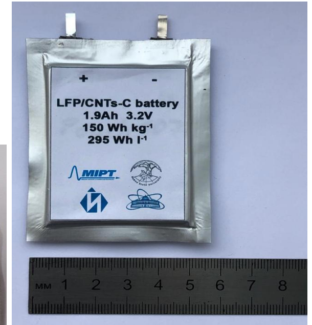
Fig 3. pouch cell after the formation and re-sealing
