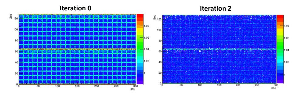
• After tower-by-tower calibration the absolute scale variation is significantly reduced
