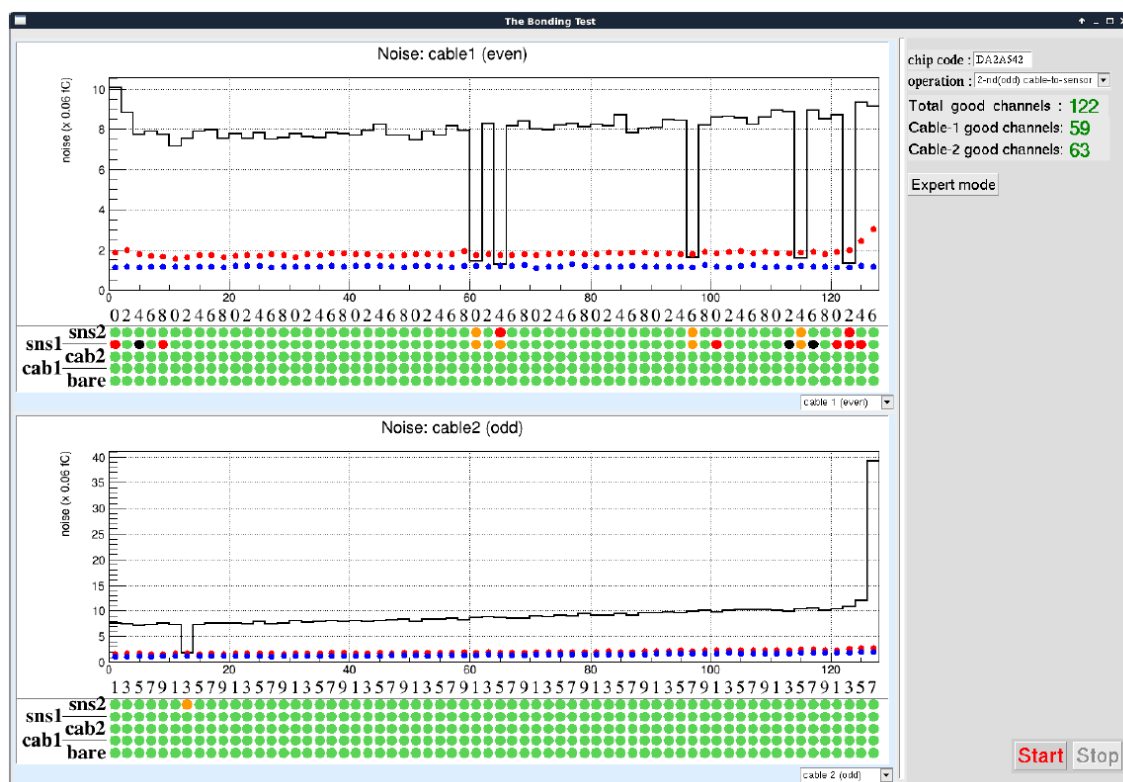
Fig. 4.9.4: GUI of the Bonding test program. Test of bondings between the ASIC 2-nd micro-cable and the sensor. Histograms of the magnitude of noise versus the channel number are
