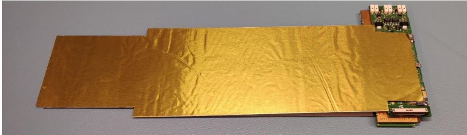
Fig. 4.2.16: Assembled STS module with shielding
