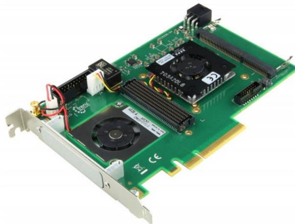
Fig. 4.4.8: TRENZ TEC0330-4 PCIe Gen2 Interface Board as best candidate for the physical interface to the computing node.
