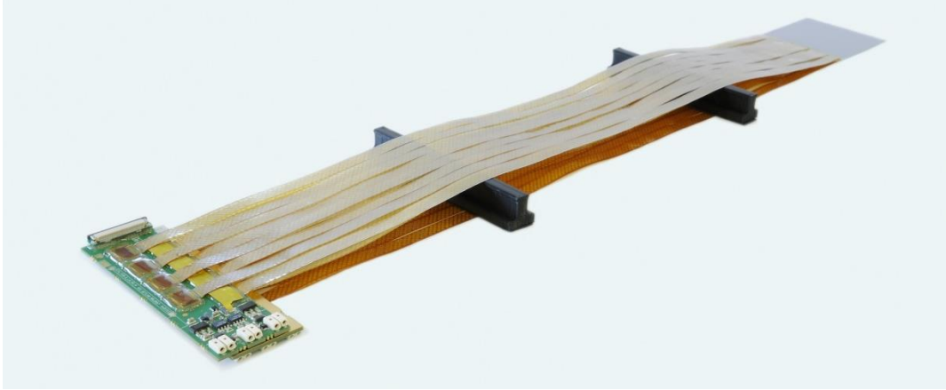
Fig. 4.4.4: Full sensor module equipped without a shielding layer to show micro-cable routing.
