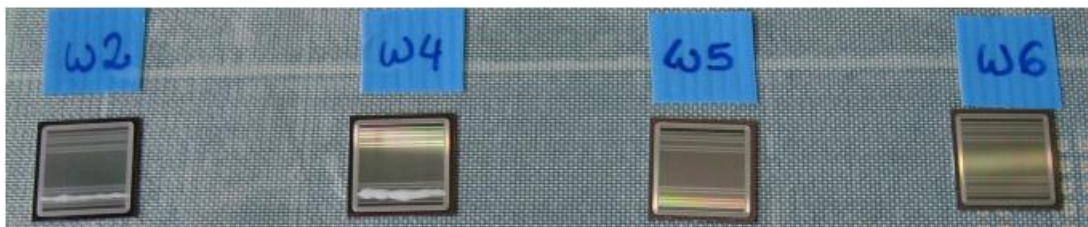
Fig. 4.6.23: prepared small sensors for irradiation test.
