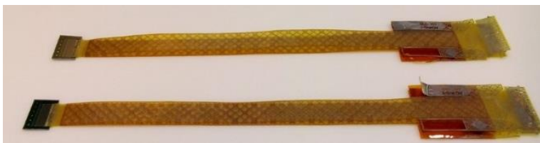
Fig.4.6.13a: ASICs with top and bottom layer micro-cables
