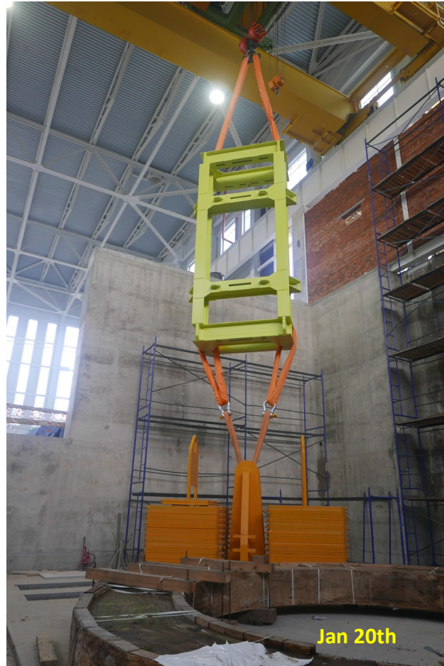
MPD Hall crane weight test
