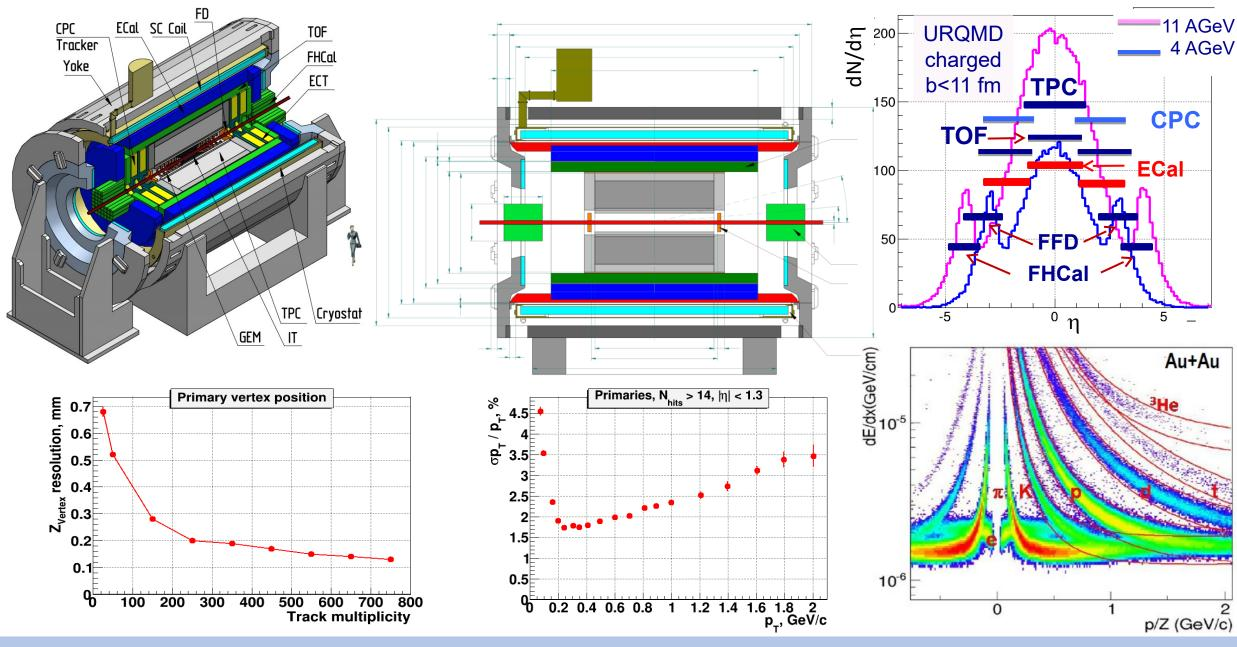
2π in azimuth, 3-D tracking (TPC), Powerful PID (TPC, TOF): - π/K up to 2.0 GeV/c, - K/p up to 3 GeV/c, Low material budget, High rate (<=6 kHz) Adam Kisiel, JINR/WUT
