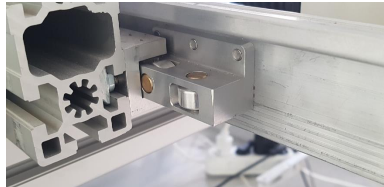
Carriages for TOF module sliding into the MPD
