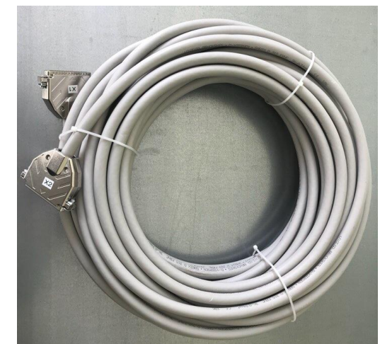
28 LV power cables needed
