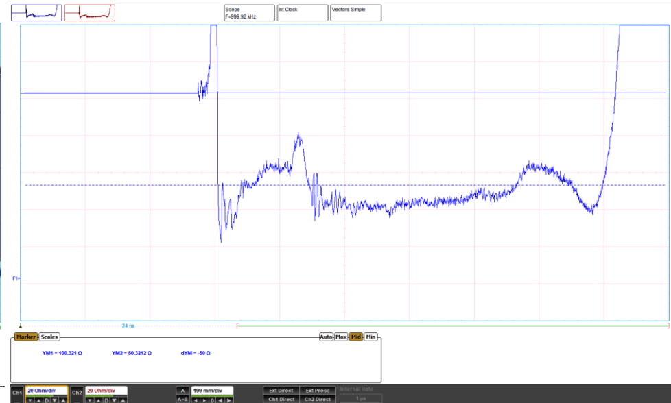
Transmission line impedance control
