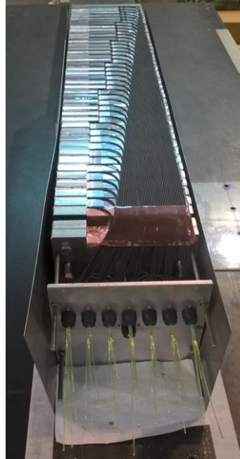
WLS-fibers are aligned.
