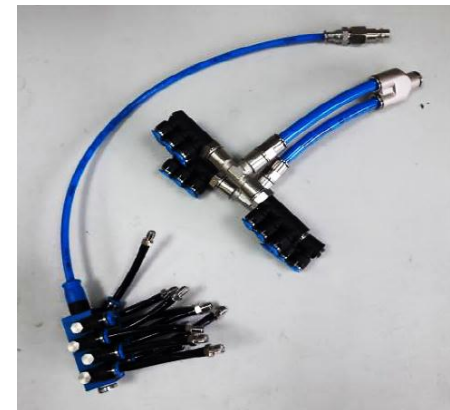
Cables and distributors of air flow to FFD modules
