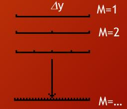
of the rapidity distribution on the size  $\delta y (\Delta y/M, M$  is the number of bins,  $\Delta y$  is the size of the mid rapidity window, N-number of particles in  $\Delta y$ ,  $k_i$ -the number of particles in bin j ):
