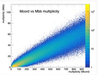
Linear relation # hits miniBeBe vs MCORD  $\rightarrow$  on-line centrality trigger?
