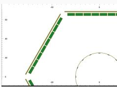
Inner detector  $\rightarrow$  miniBeBe cylinder [71.4 cm length, 52 cm diameter]
