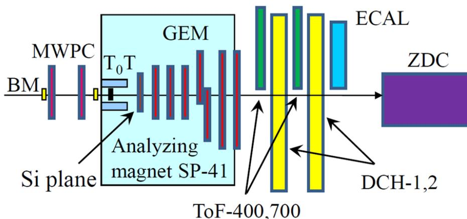
Figure 1: Scheme of the BM@N set-up in the carbon beam run.
