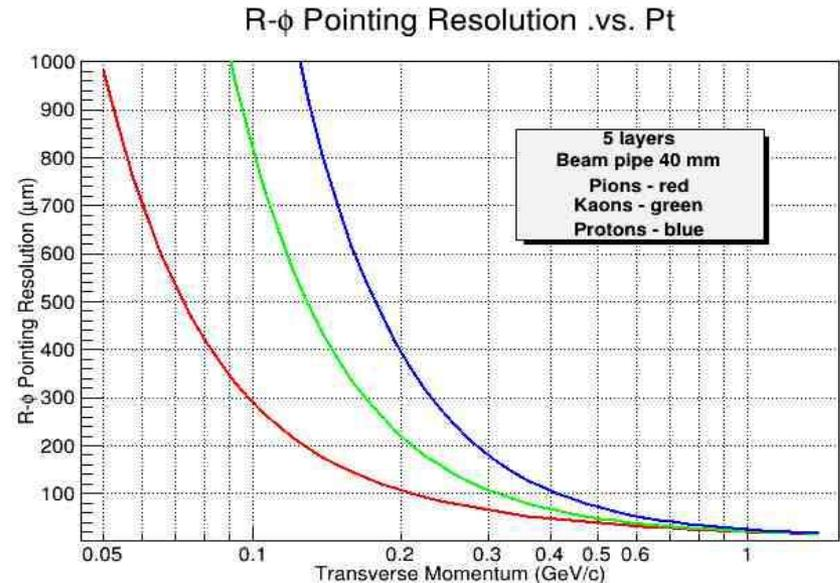
Evaluated resolution of IT5-40 provides, for example, the possibility of  $D^0$  decay vertex reconstruction in the channel  $D^0 \rightarrow K^- + \pi^+$  ( $\lambda = 123 \mu\text{m}$ ) with small  $p_T$  up to 300 MeV/c.
