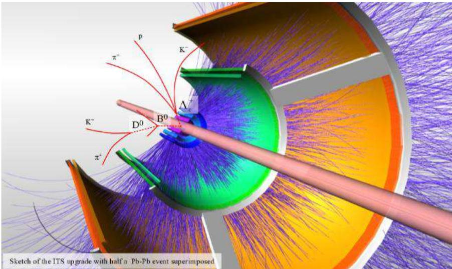
Modern vertex detectors consist of a few layers of **silicon position-sensitive sensors**.
