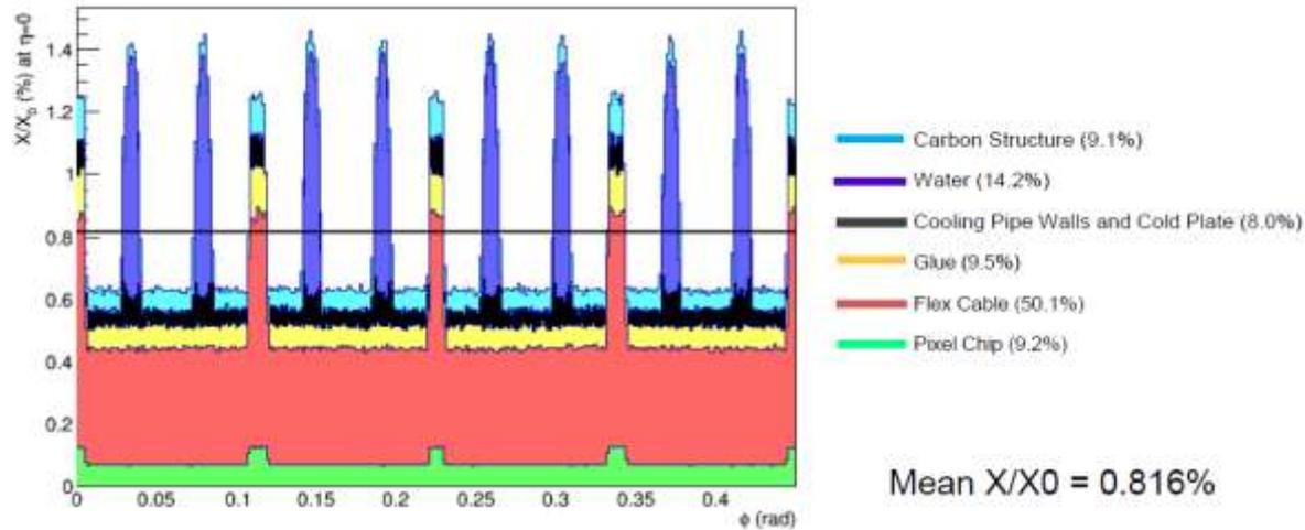
Effective Si thickness  $t=760 \mu\text{m}$
