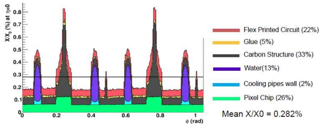
Effective Si thickness  $t=260 \mu\text{m}$
