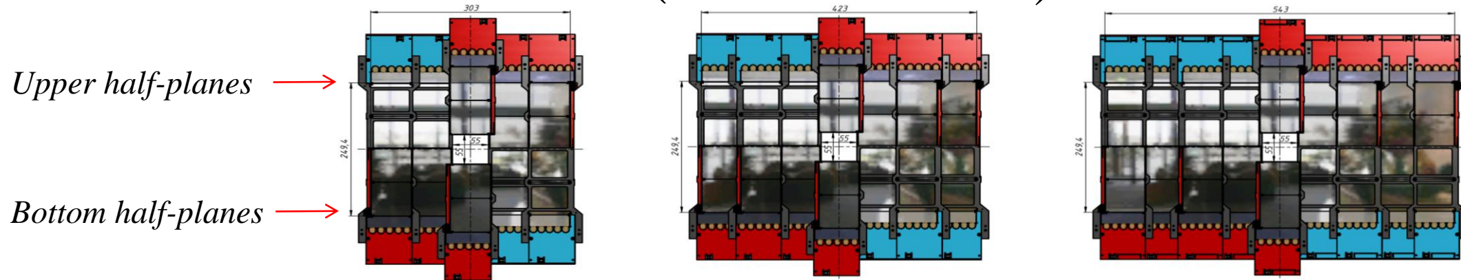
Three tracking silicon planes with FEE boards (using only one type of Silicon Detector Module!)
