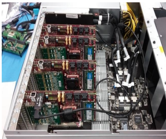
Compute node with data processing boards
