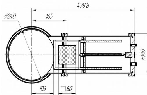
*Tentative design (by BSU Group) of moving mechanics for Si Beam Profile Detectors*
