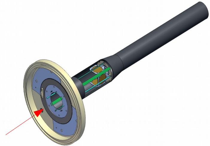
Carbon vacuum pipe and the target station
