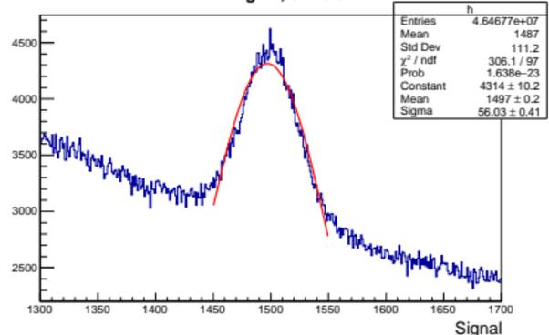
Embedded signal for SILICON part of the tracker looks wider (if comparing with GEM) due to more significant fluctuations of Command Mode when decoding
