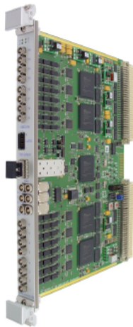
Figure 5: Image of the 16 channel, 250 MHz, 14 bit digitizer module SIS3316 from Struck [24].
