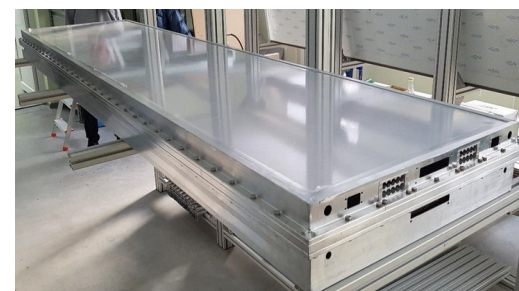
Automatic painting of the conductive layer on the glass
