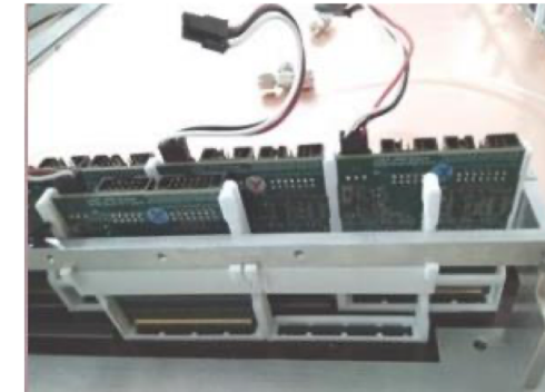
New bracing system for FEE was designed and produced
