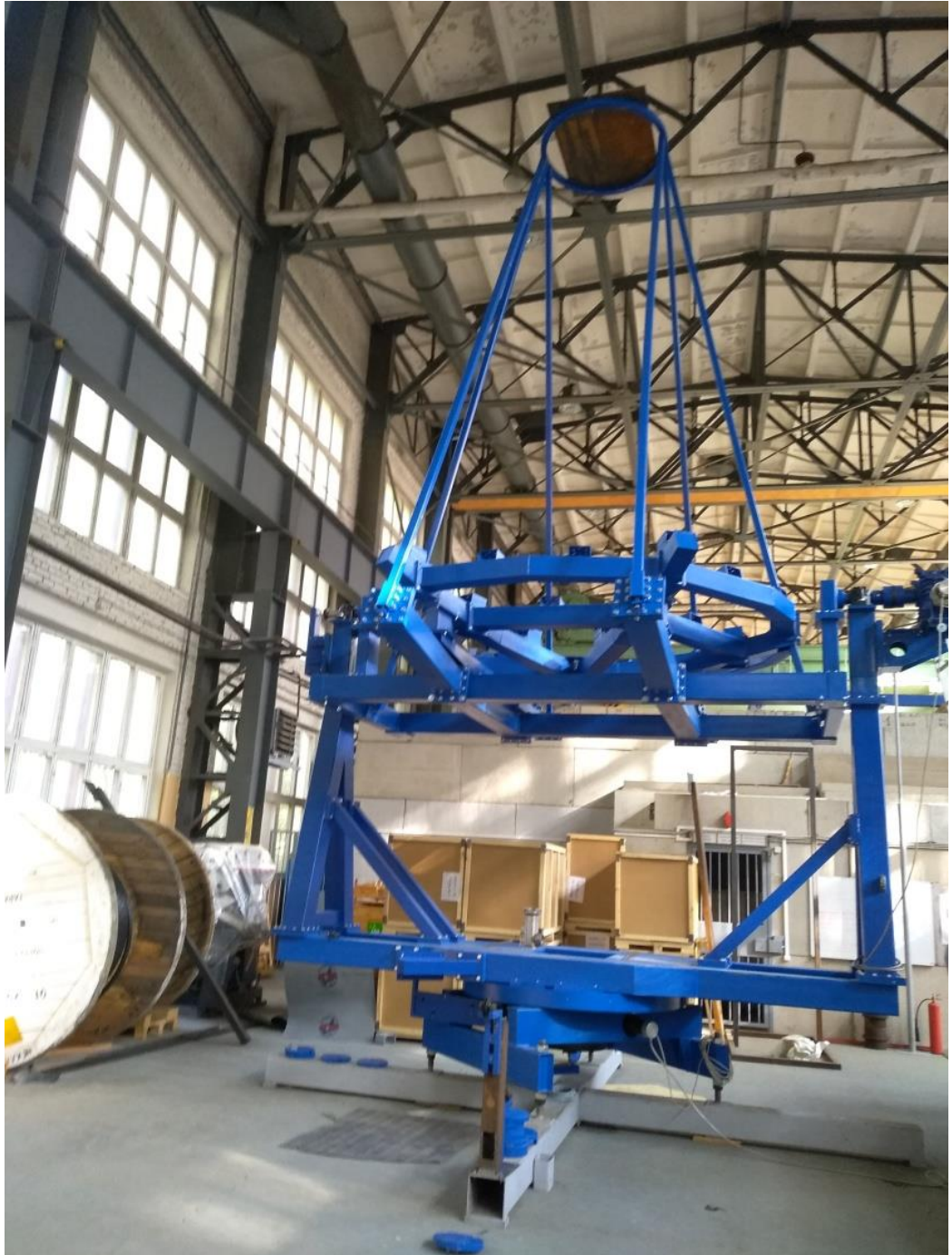
Fig.4. IACT#3 mounting in assemble at JINR workshop
