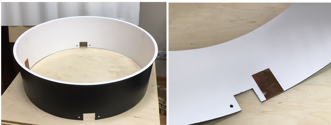
Figure 35. The additional element of the EMFS. In the second photo one can see the electrical contact of the rf-screen. The main element has the same contact too.
