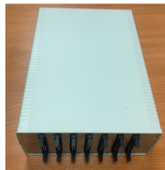
a) - Custom made HV unit by JINR
