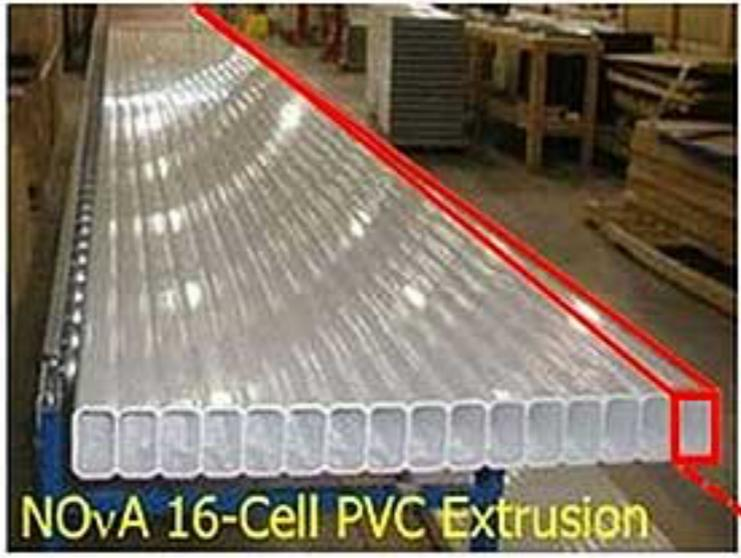
NOvA 16-Cell PVC Extrusion
