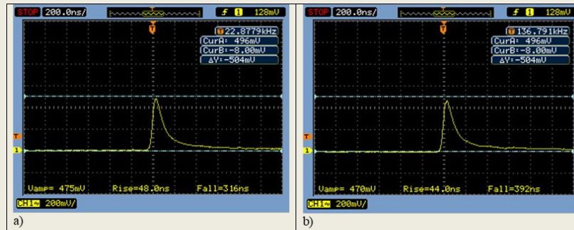
Fig.9 Average strip signals for (a) 70 kHz and (b) 250 kHz strip r/o channel loads
