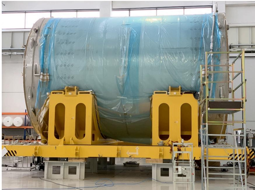
*Fig.3.2.2 . Completely built solenoid.*
