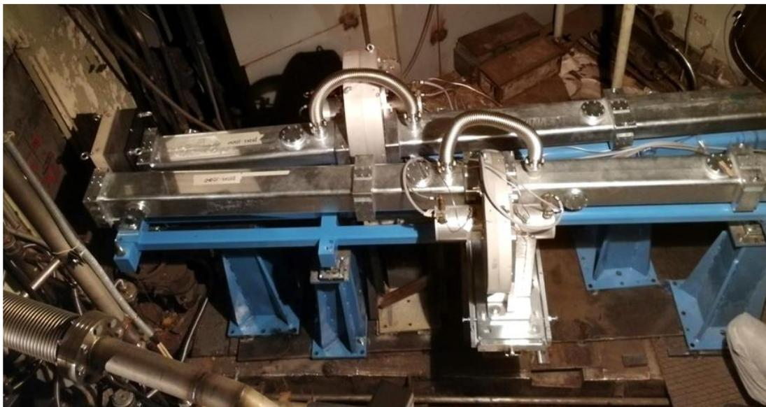
**Fig. 44.** A new head part of channel 10 in the ring corridor of the IBR-2 reactor, consisting of two neutron guides and double-disk background choppers installed in the corresponding technological gaps.
