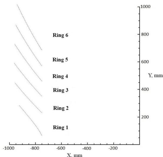
**Fig. 7.** Shape of the detector elements of the rings.
