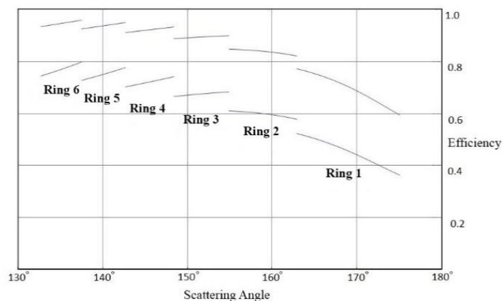
**Fig. 6.** Dependence of the detector efficiency on the scattering angle.
