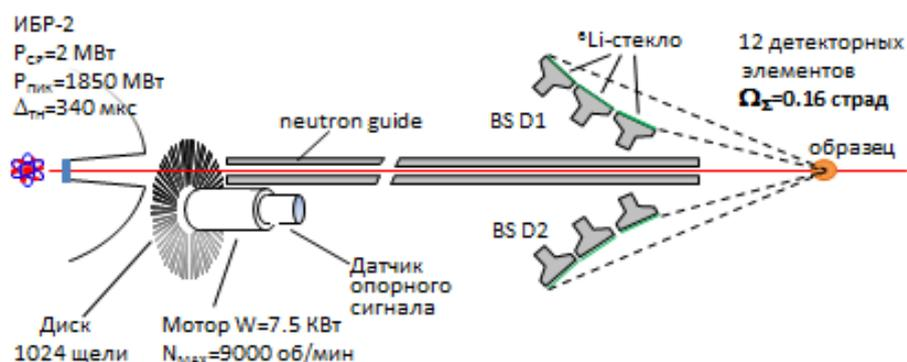
**Fig. 1.** Layout of HRFD at the IBR-2 reactor.
