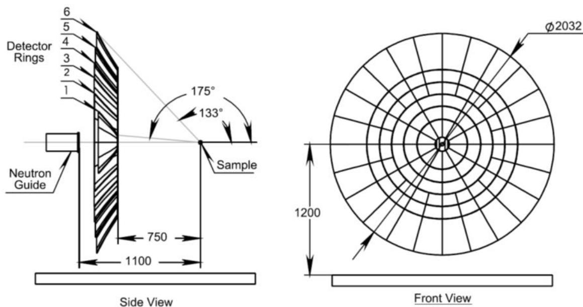
**Fig. 2.** Schematic of the large-aperture backscattering detector.
