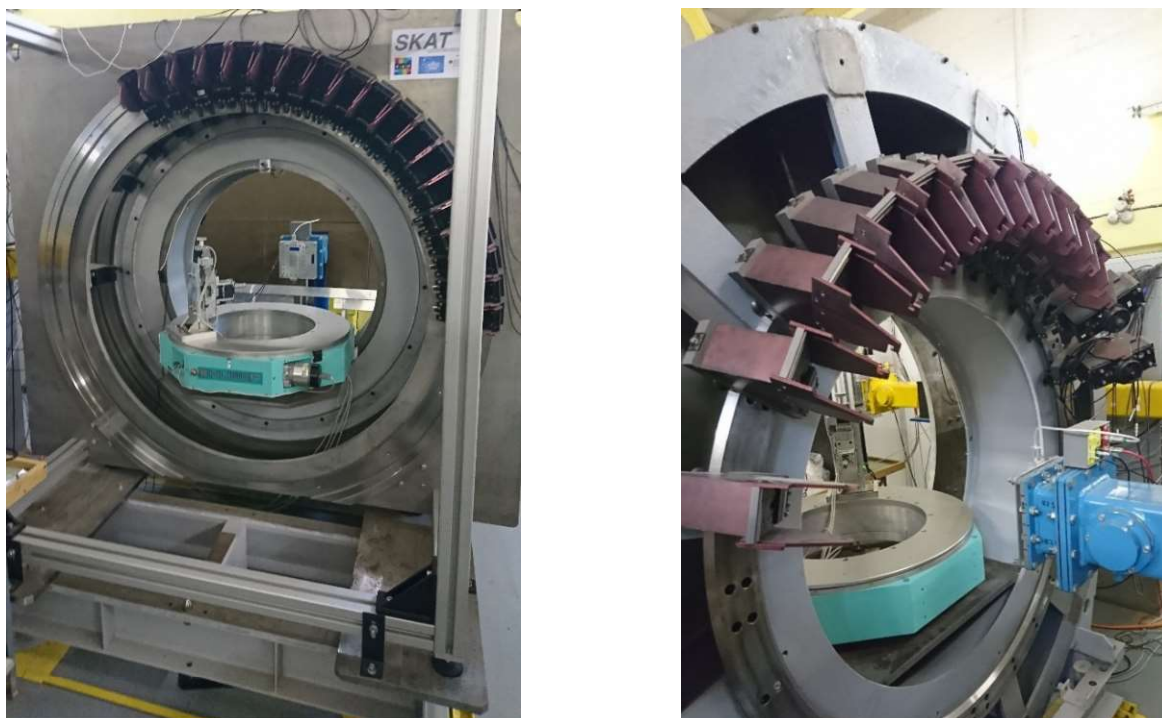
Fig. 17. Currently available mounting places for detectors at scattering angles 2\theta = 65^\circ (left) and 2\theta = 135^\circ (right) at the SKAT diffractometer.
