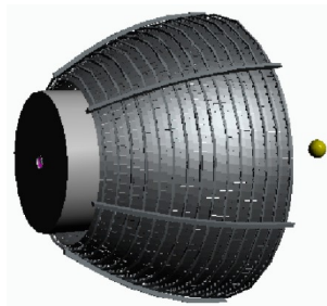
Fig. 27. The geometry of the new INS spectrometer with inverse geometry: a) general layout; b) two symmetric parts of the spectrometer with pyrolytic graphite analyzers; c) one part of the spectrometer with beryllium filter and detector.
