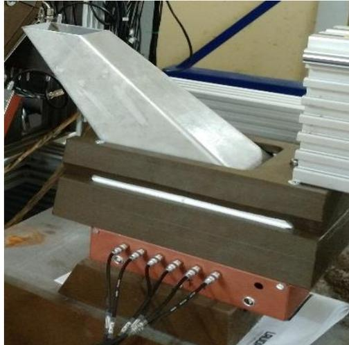
**Fig. 18.** Module of 45° ring detector for the DN-6 spectrometer.
