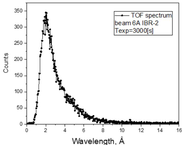
**Fig. 24.** Time-of-flight spectrum measured for 3000 s (the figure shows the Maxwell distribution of the neutron flux as a function of the wavelength).
