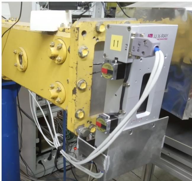
**Fig. 29.** “JJ X-RAY” slit system at the FSD diffractometer.
