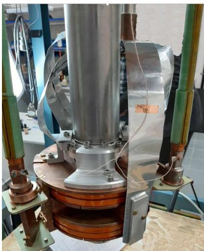
**Fig. 7.** HTSC magnet and current leads.
