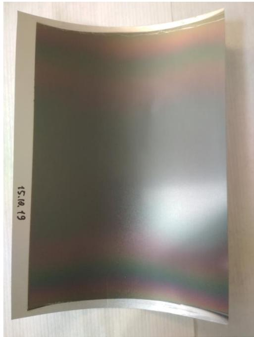
**Fig. 16.** Specimen of sputtered B<sub>4</sub>C film on aluminum substrate (film thickness in the central part – 2 μm).
