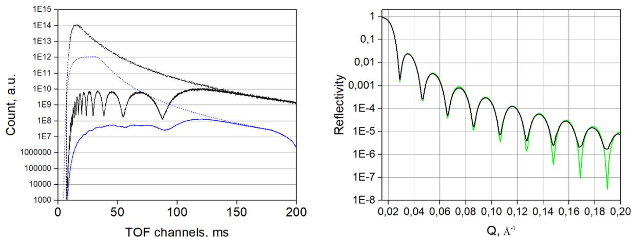
**Fig. 6.** Left: TOF spectra of direct and reflected beams for two sources separately. Blue – delayed neutrons, black – neutrons from a pulsed source. The dotted line corresponds to direct beams, the solid line – reflected beams. Right: reflectivity curves with (black) and without (green) background source.
