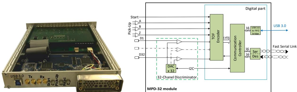
**Fig. 26.** MPD32-USB3 data acquisition module (left – prototype, right – block diagram).
