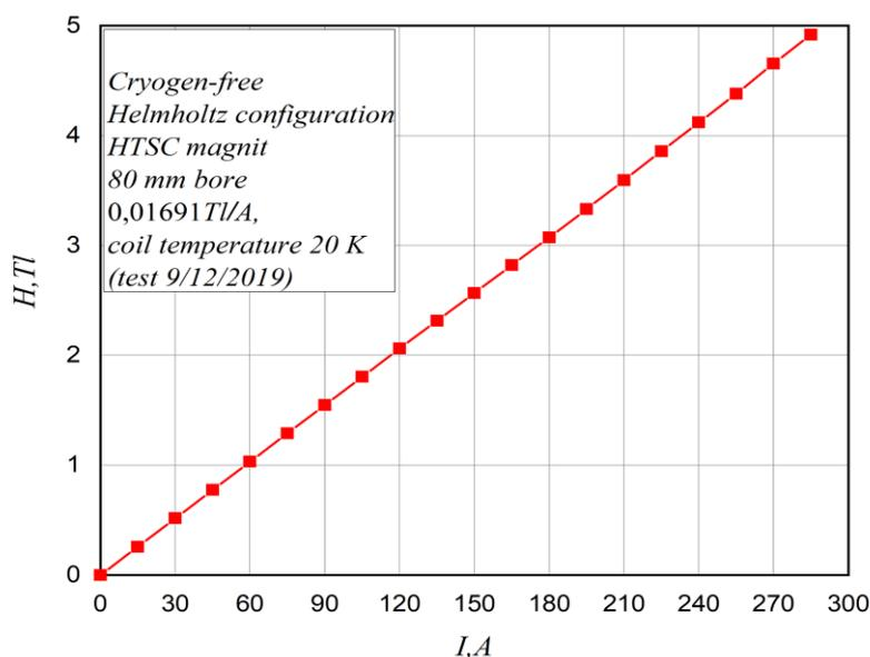
**Fig. 8.** Dependence of the magnetic field strength on the magnitude of electric current supplied to the magnet coils (this characteristic turned out to be strictly linear, which indicates that there are no signs of degradation of the HTSC tape).
