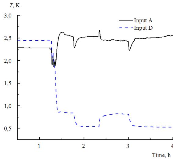
**Fig. 10.** Switching from the continuous mode to the single mode and back (temperature of the evaporator varies from 0.78 K to 0.52 K). Input A - temperature of the second stage of the cryocooler. Input D is the evaporator temperature.
