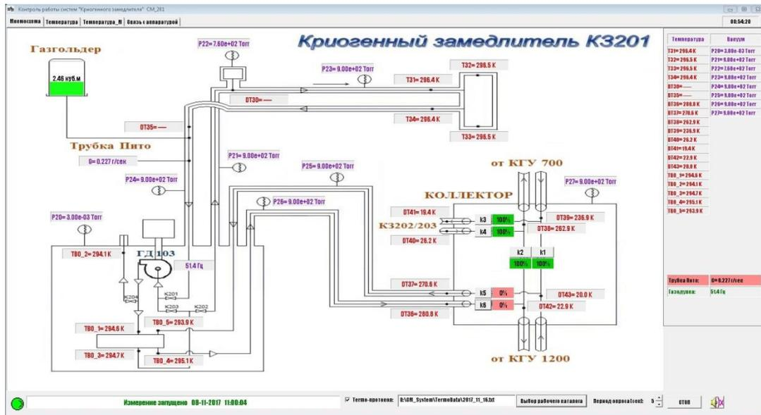
Fig. 2. Control program for the CM-201 pelletized cold moderator.
