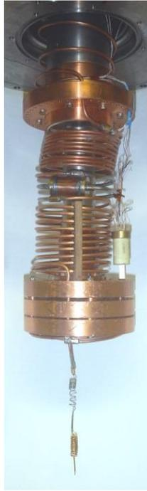
**Fig. 9.** Refrigerator with a continuous flow system of heat exchangers.
