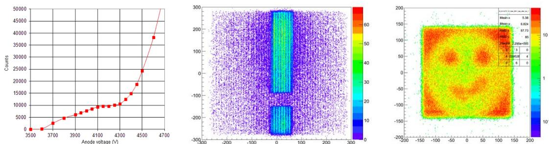
**Fig. 17.** Left: counting characteristics at 2000 mbar of CF<sub>4</sub>. Middle: direct beam of IBR-2 beamline 13 with a 1-cm cadmium plate (channel graduation – 0.194 mm). Right: spectrum from a scattered neutron beam covered by a cadmium mask (channel graduation – 0.388 mm).
