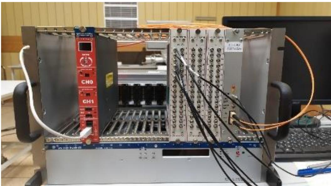
**Fig. 19.** 96-channel data acquisition system for the DN-6 spectrometer.
