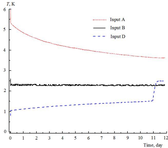
**Fig. 11.** Mode with a zero external-pumping rate: the temperature of the evaporator rises slowly from 1.05 K to 1.5 K in the period of 0-11 days, then increases sharply to 2.7 K and stabilizes at this level (Input A – temperature of heat exchangers; Input B – temperature of the second stage of the cryocooler; Input D – temperature of the evaporator).
