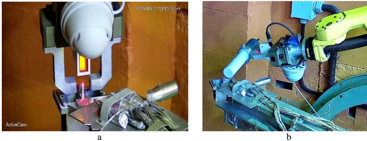
**Fig. 4.** Photos of the robotic arm taken using one of the cameras of the video surveillance and distance measuring system: **a** – pneumatic clump of the robotic arm at the moment of removing the container with a highly radioactive sample; **b** – dose measurement using the local dosimetry system at the moment before the robotic arm removes the container with the sample (radiation dose rate on the surface of the container  $\sim 78$  mSv/h).
