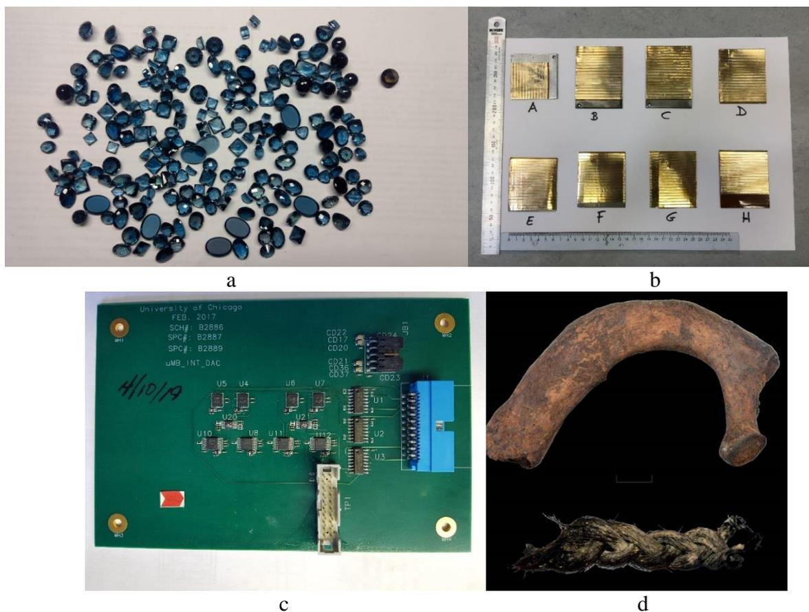
**Fig. 5.** Samples after irradiation on beamline 3 of the IBR-2 reactor: **a** – samples of topazes; **b** – detector materials; **c** – electronic components of printed circuit boards; **d** – fragments of the remains of members of Tsar Ivan the Terrible’s family.
