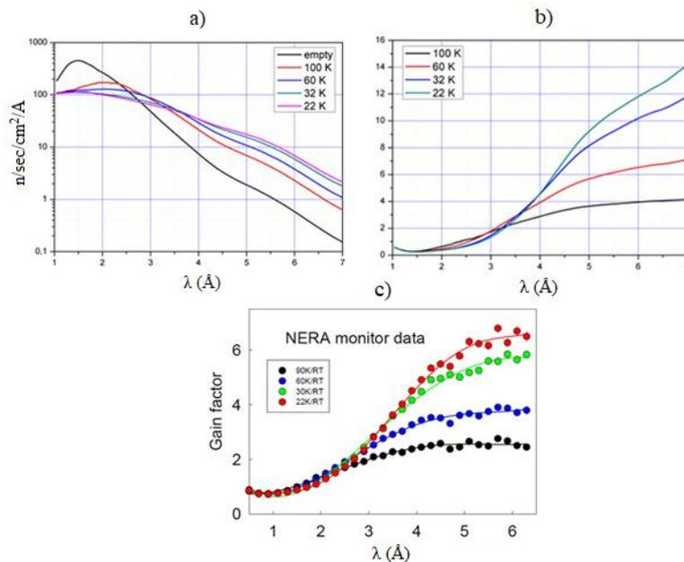
**Fig. 3.** Neutron spectra (a) and gain factor (b, c) in the cold neutron flux density from the surface of the cold moderator at different temperatures as compared to the cold neutron flux density from the surface of the thermal room-temperature water moderator. The graphs in figures *a* and *b* were obtained with the REMUR reflectometer, and in figure *c* – with the NERA spectrometer.
