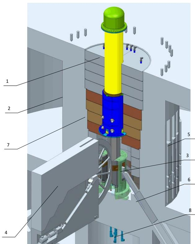
**Fig. 1.** The NEPTUN reactor in mass concrete: 1 – reactor vessel; 2 – mass concrete; 3 – stationary reflector; 4 – reactivity modulator; 5 – neutron beam shutters; 6 – technological part of the moderator; 7 – thermal shield; 8 – drives of control and protection system units.
