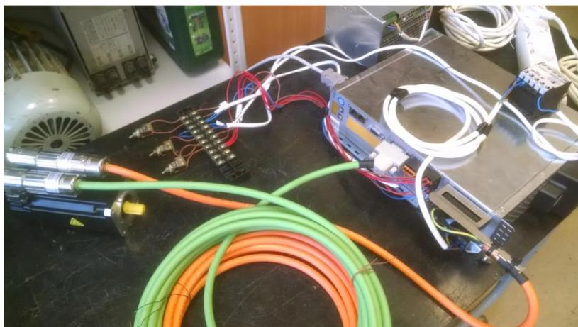
**Fig. 28.** Test stand “motor – servo-amplifier”.
