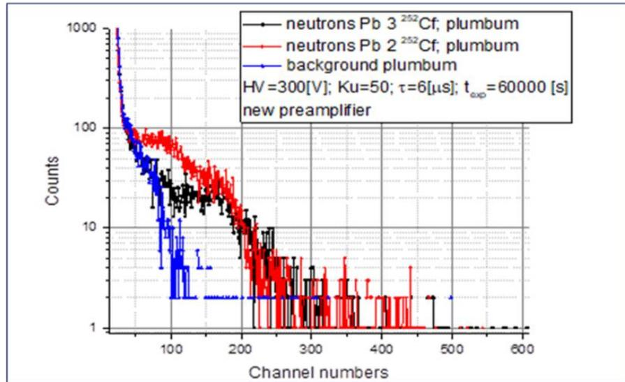
**Fig. 22.** Amplitude neutron spectra obtained with a <sup>252</sup>Cf source (high voltage  $H_v = 300$  V, signal shaping time  $\tau = 6 \mu\text{s}$ , gain  $K_U = 50$ , measurement time  $t_{\text{exp}} = 60,000$  s, gamma radiation shielding – lead plate 0.5 cm thick).
