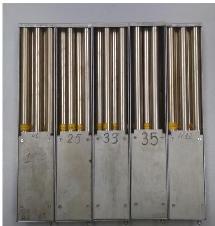
**Fig. 15.** Variants of the detector modules for the NERA spectrometer, ready-assembled with a preamplifier and interference shielding.
