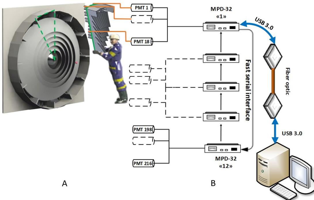
**Fig. 25.** A scale model of BSD (A) and the architecture of the data acquisition system (B).
