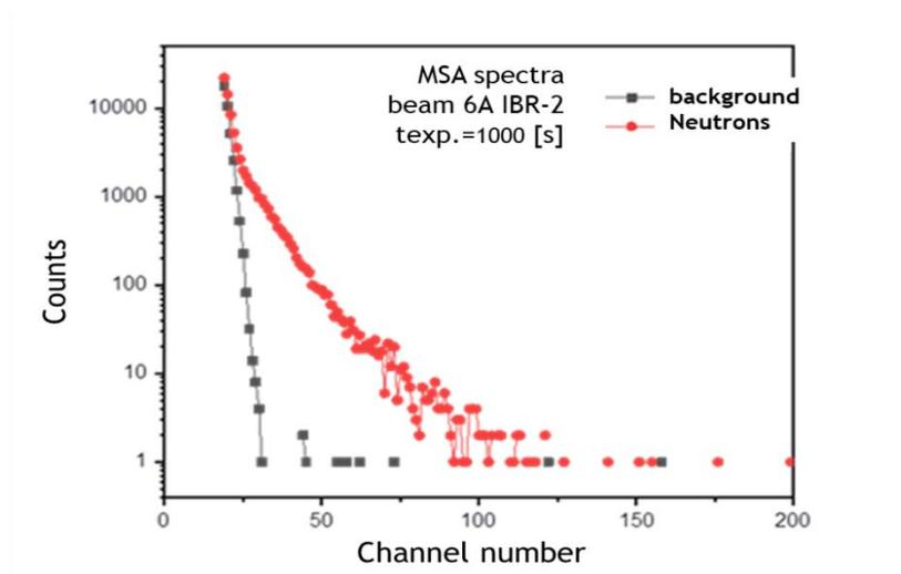
**Fig. 23.** Amplitude spectra of  $\text{LiInSe}_2$  measured in a direct beam of IBR-2 beamline 6a (voltage – 300 V, measurement time – 1000 s).
