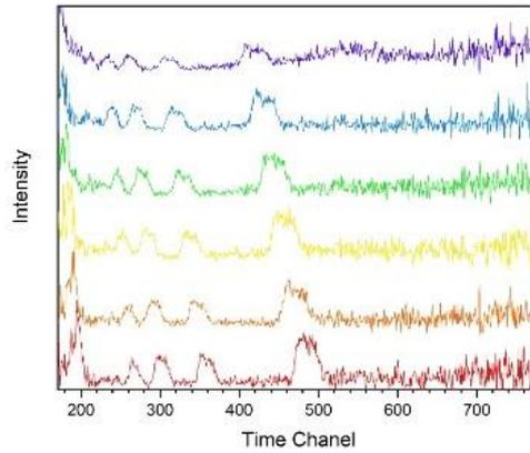
**Fig. 20.** TOF spectra obtained from one module of 45° ring detector.
