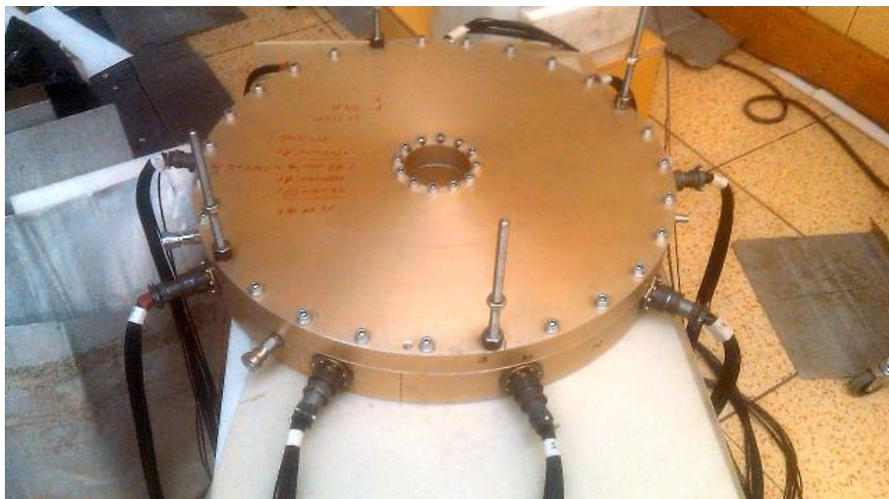
**Fig. 13.** Photo of the ring-shaped multi-section detector on a test stand.
