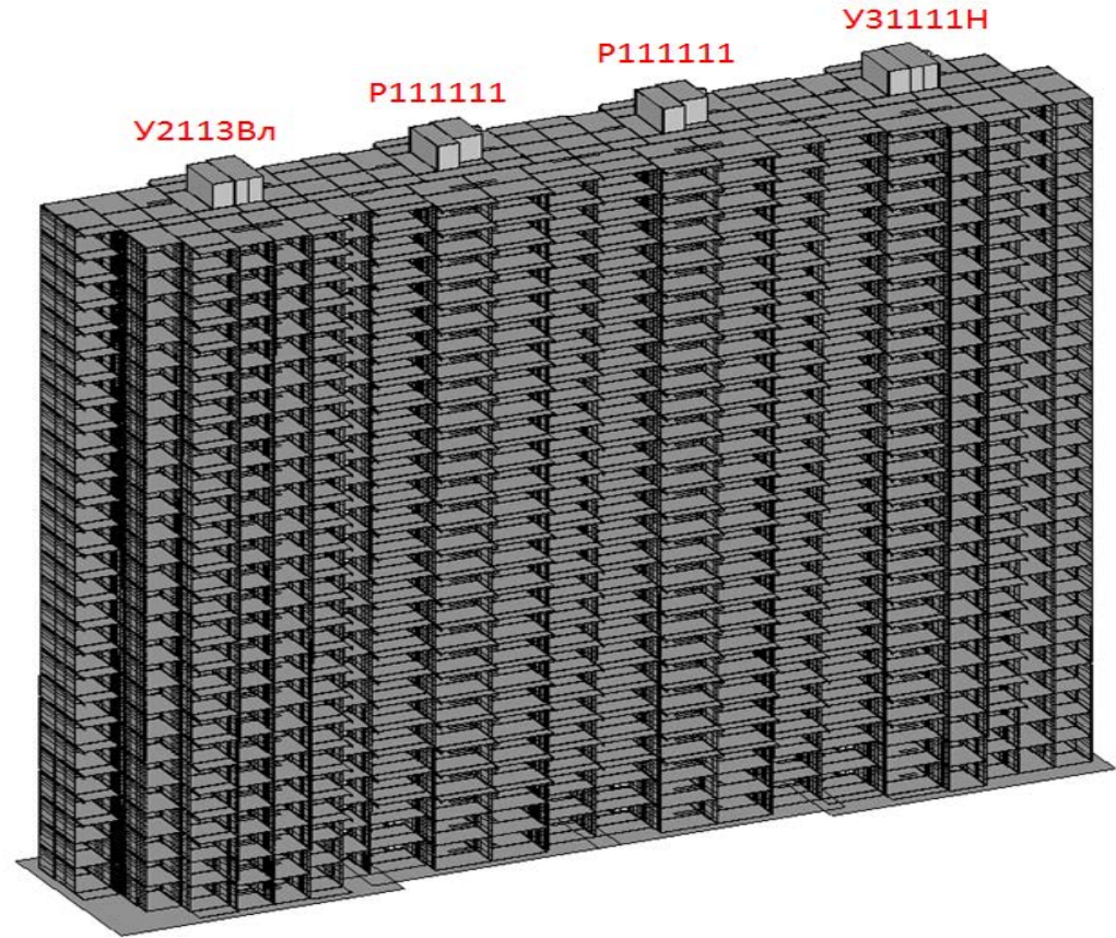
Isometric views of finite element model of temperature block from 4 modules
