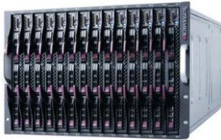
SuperBlade Chassis including 10 calculation blades for run user tasks.
