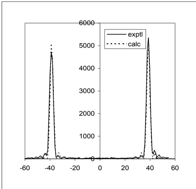
Phase matching SHG angles correspond to unperturbed director alignment ( $0^\circ$ ), i.e., significant part of LC is not effected by electric field
