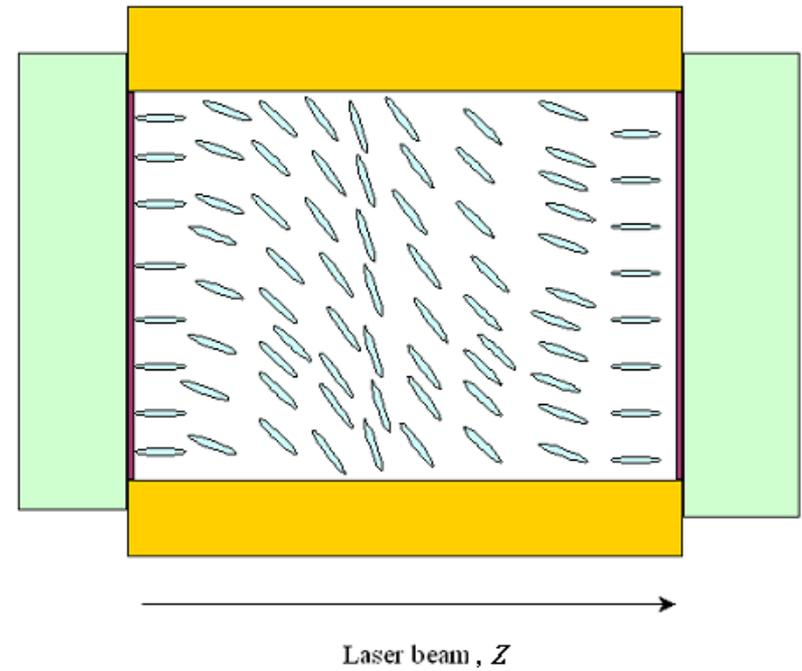
One-dimensional case solution. There are smooth changes of deformation angle. No layers and no borders between layers. Most part of the LC is effected by electric field.
