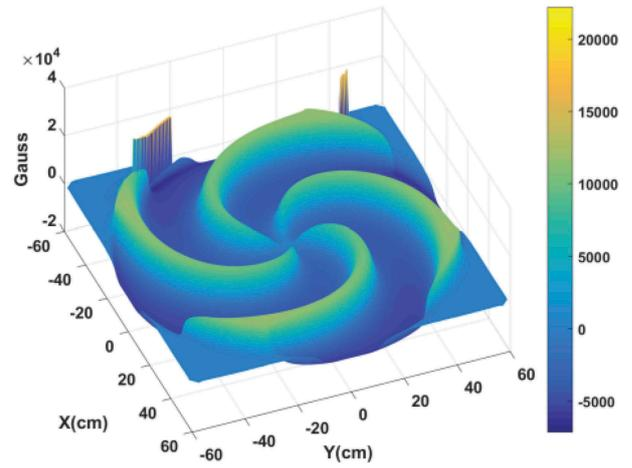
**Figure 1.** Overview of the flutter field of the SC200 cyclotron.
