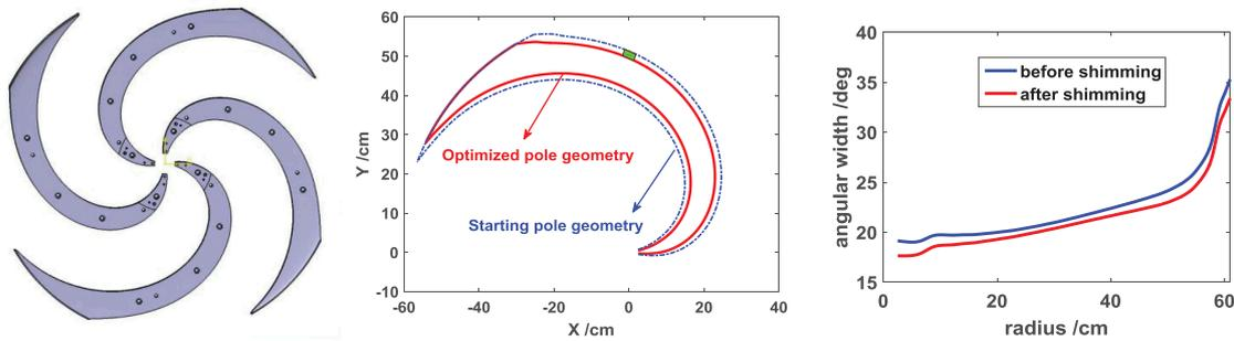
**Figure 9.** Overview of the pole structure for SC200 (left), starting and optimized pole geometry (middle), and the angular width of the poles before and after shimming (right).
