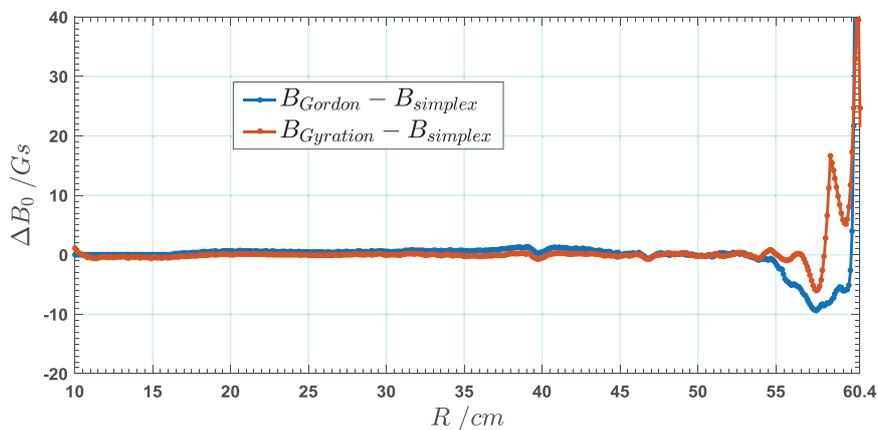
**Figure 5.** Difference between the isochronous field obtained from Gordon's method, the gyration frequency-based method, and the 12<sup>th</sup>-order simplex method.
