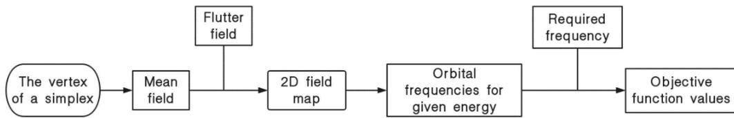
**Figure 3.** Flow chart for calculating the objective function.
