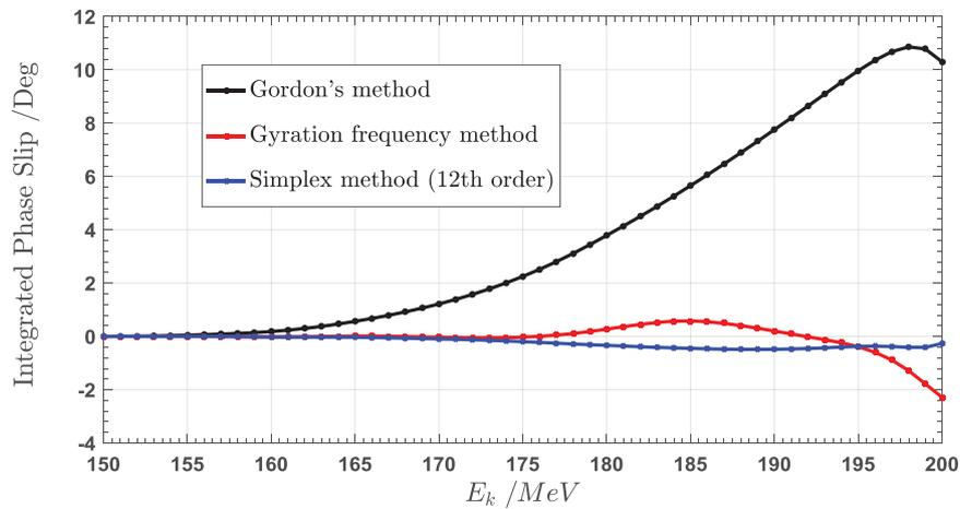
Figure 7. Comparison of the integrated phase slip during acceleration from 150 MeV to 200 MeV.
