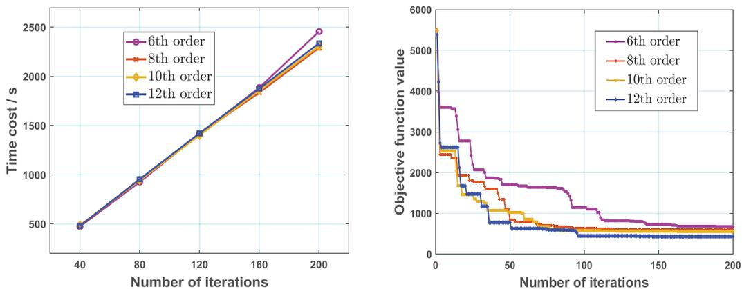
Figure 8. Time cost for different-order simplex methods (left), and the value of the objective function for different-order simplex methods during the iterations (right).
