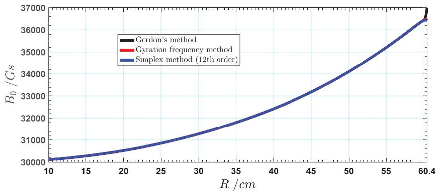
**Figure 4.** Comparison of the isochronous field obtained from Gordon's method, the gyration frequency-based method, and the 12<sup>th</sup>-order simplex method.
