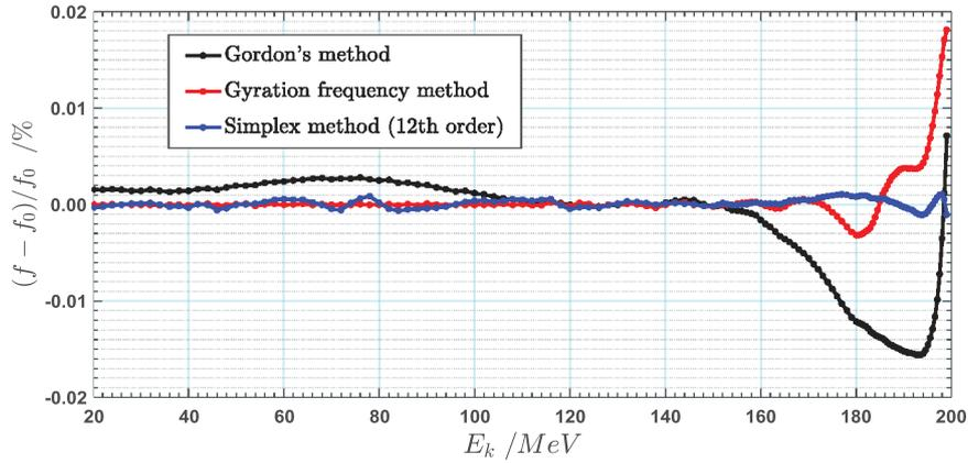
Figure 6. Relative error in the orbital frequency of Gordon's method, the gyration frequency-based method, and the 12<sup>th</sup>-order simplex method.
