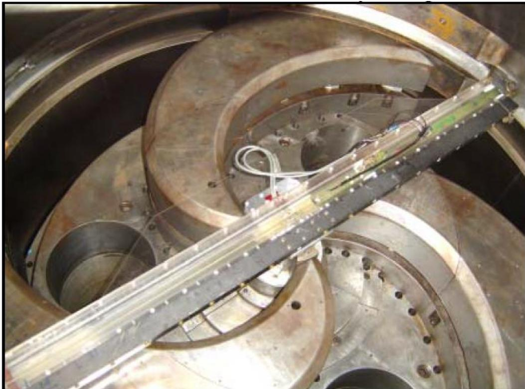
Figure 45:VECC Kolkata cyclotron magnetometer with inductive coil.
