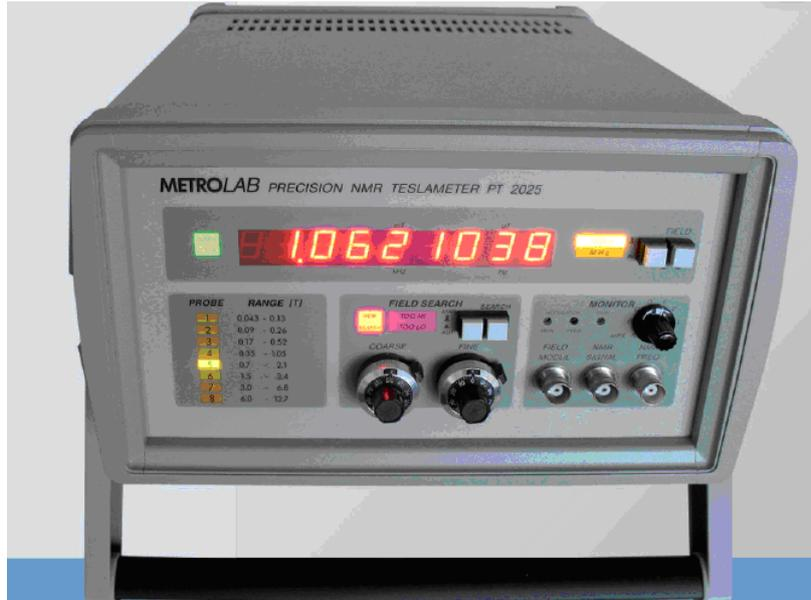
Figure 44: Metrolab NMR teslameter PT2025 (FLNR has one).
