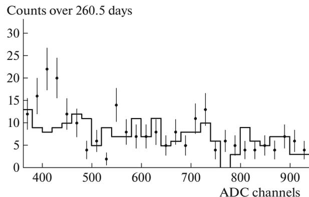
**Fig. 3.** Delayed events detected by the NaI(Tl) detector when measuring the background. The channel range of 380–460 corresponds to the energy of 137 keV. Dots with errors indicate events with a sampling window of 1.8–5.0  $\mu\text{s}$ . The solid line shows the delayed coincidences with a window of 11.8–15.0  $\mu\text{s}$ .
