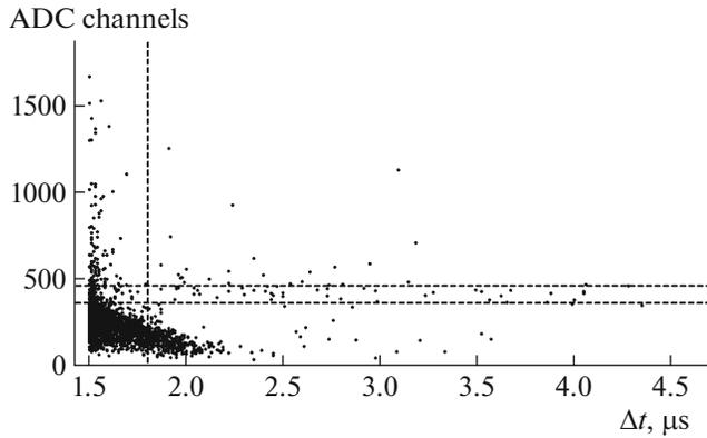
**Fig. 1.** Delayed events (dots) detected by the NaI(Tl) detector in the presence of a neutron source: ( $\Delta t$ ) delay time. The dashed line indicates the region of interest in the range from 1.8 to 5.0  $\mu\text{s}$ . A large number of events below the region of interest are the afterpulses of the photomultiplier tube.
