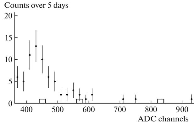
**Fig. 2.** Delayed events detected by the NaI(Tl) detector over 5 days of measurements in the presence of a weak neutron source. Dots with errors indicate events with a sampling window of 1.8–5.0  $\mu\text{s}$ . The solid line shows the delayed coincidences with a window of 11.8–15.0  $\mu\text{s}$ . The channel range of 380–460 corresponds to the energy of 137 keV.
