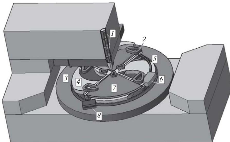
**Fig. 1.** Computer model of a compact cyclotron: (1) solenoids, (2) harmonic coils, (3) main winding, (4) sector forming magnetic field, (5) electrostatic deflector, (6) magnetic channel, (7) accelerating dees, (8) corrector of magnetic field decline.
