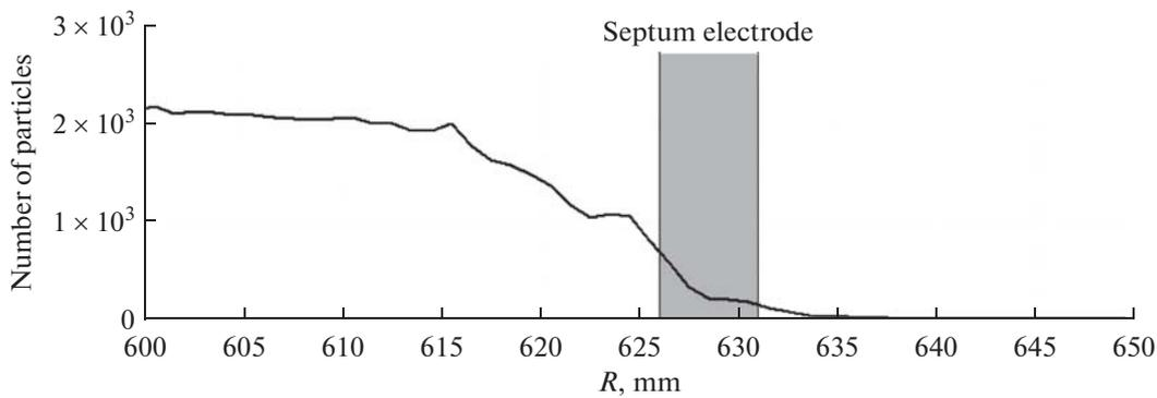
Fig. 6. Choice of position of electrostatic deflector septum on the basis of values of differential probe.
