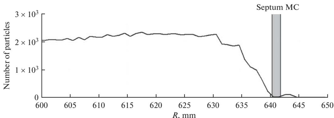
Fig. 7. Choice of position of magnetic channel septum on the basis of values of differential probe.
