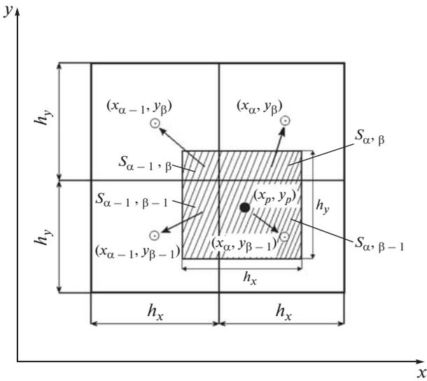
**Fig. 5.** Initial kernel of PIC model. Interpolation scheme of transferable factor to Euler grid.
