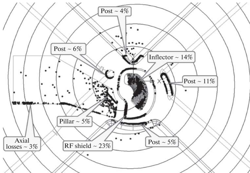
**Fig. 8.** Graphical representation of distribution of lost particles in central domain of compact cyclotron. Black spheres are lost particles.
