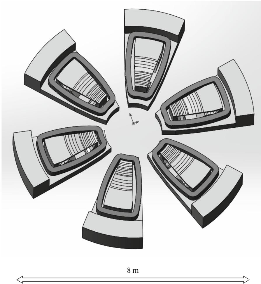
Fig. 8. Magnetic system of the booster cyclotron with a field level of 1.6 T.
