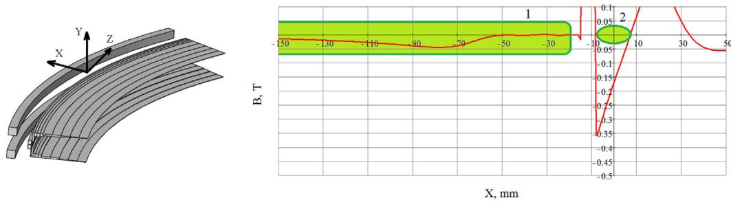
Fig. 11. Configuration of the 1st magnetic channel and its field contribution: 1 — circulating beam, 2 — extracted beam.
