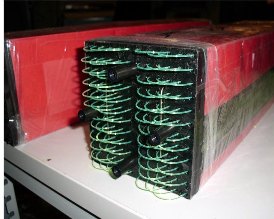
We used Y11-200 WLS fibers with multi-cladding of 1 mm in diameter.
