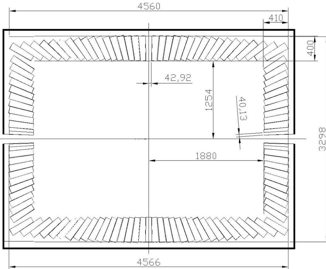
ECAL consists of trapezoidal ( $\sim 2^0$ ) cells:
