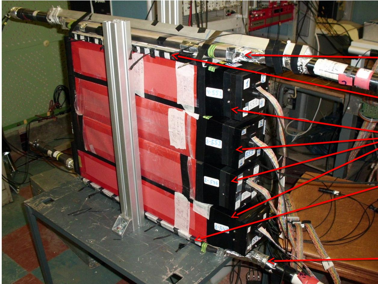
Trigg. Counter with double side readout
