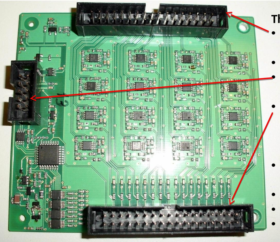
This board controlled of 16 MPPC H/V :
