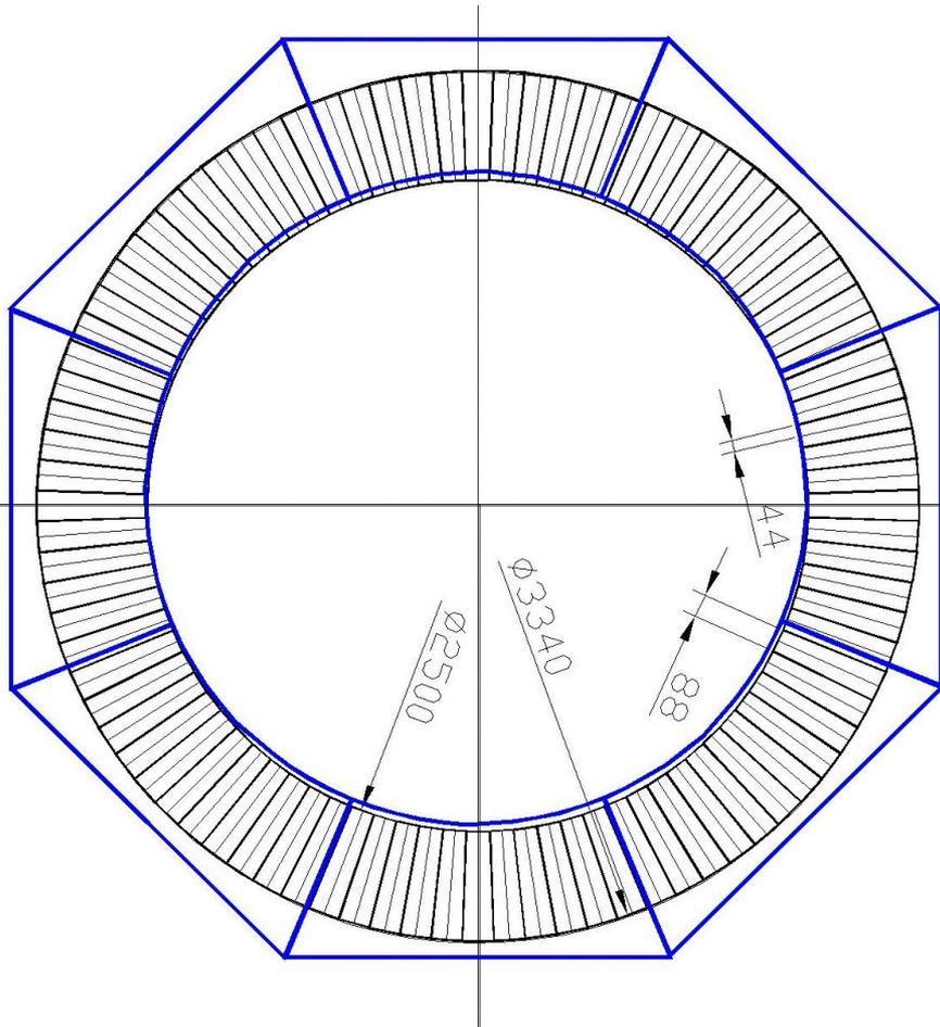
Barrel part is divided into 8 sectors of  $45^\circ$
