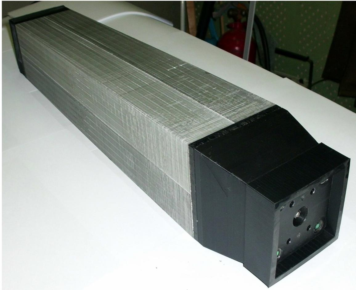
Module has trapezoidal shape with angles of about  $2^\circ$  and consists of 4 cells  $\sim 50 \times 50 \text{ mm}^2$ .
