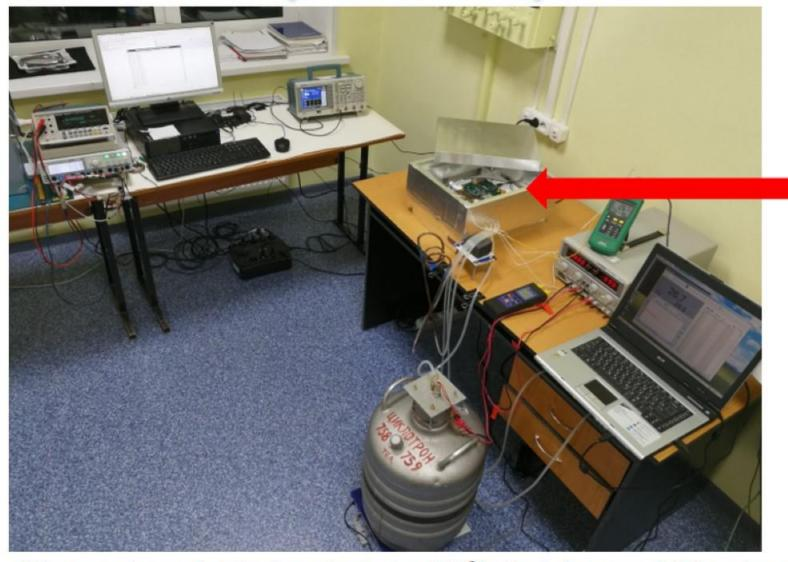
Allows us to cool detectors down to -120°C. By using an additional module it is also possible to heat detectors up to +60°C.
