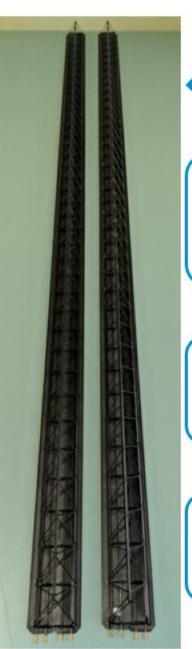
The first samples for the ITS MPD have already been constructed.
