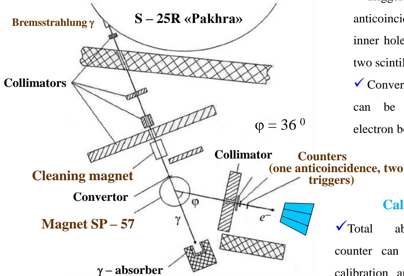
✓ Trigger signal : one anticoincidence counter with inner hole ( $d = 10$  mm) and two scintillation counter
