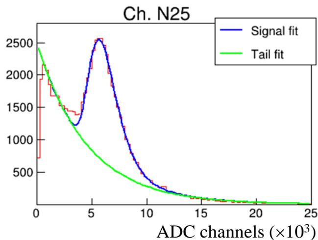
✓ Clear peak from muons can be a reliable tool for calibration
