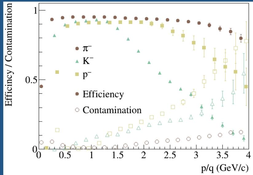
$$\text{Eff.} = \frac{\text{particles which are correctly identified}}{\text{all particles of a given species (PDG)}}$$
