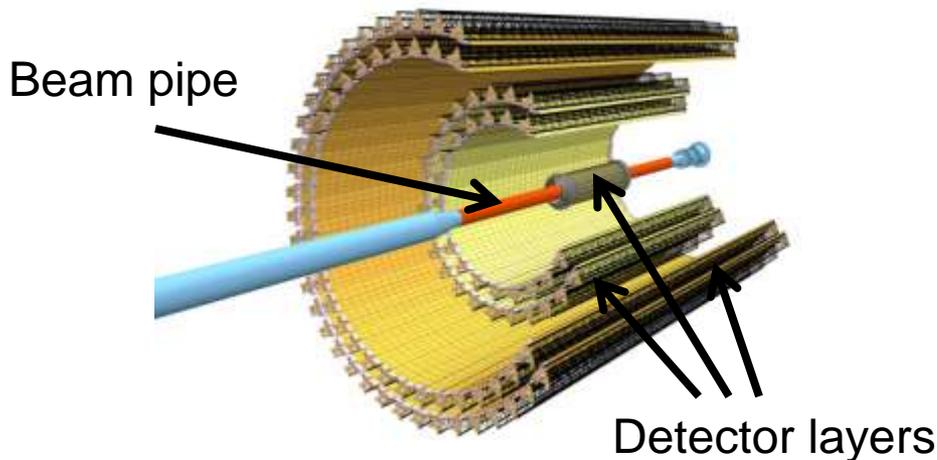
Modern vertex detectors consist of several layers of silicon position-sensitive sensors, surrounding a beam pipe. This kind of detectors are already used in ALICE , ATLAS, CMS and STAR experiments.
