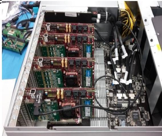
**Compute node with data processing boards**
