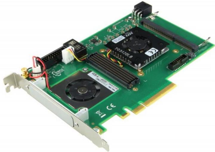
**TRENZ TEC0330-4 PCIe Gen2 Interface Board**
