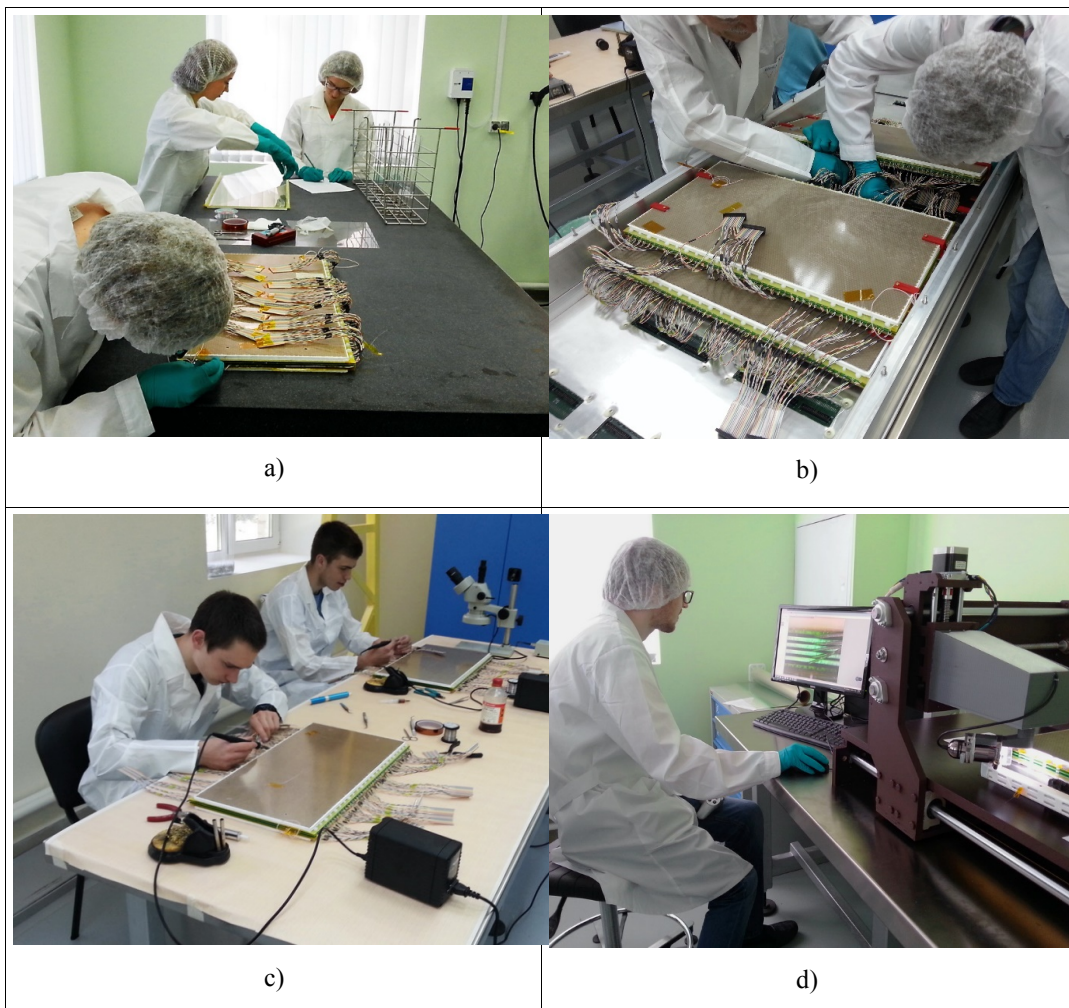
Figure 4: a) MRPC assembling process; b) TOF module assembling; c) Soldering of the signal cables; d) Control of MRPC quality and uniformity of gaps.
