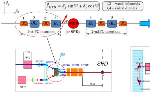
The collider lattice fragment where weak "navigator" solenoids are installed
