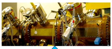
• The RFQ, put limit for proton energy - 5 MeV at the linac LU-20 output (instead of 20 MeV ). The new proton and light ion linac "LILAC" is now manufacturing . The LILAC output energy is 12 MeV.
