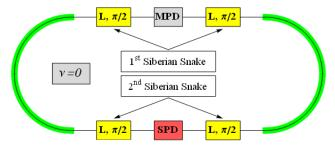
$\Psi$  — angle between the polarization and the particle velocity. The field integral of 0,6 T·M, provides  $\Delta v = 0.01$  for protons and  $\Delta v = 0.003$  for deuterons. Minimum spin reversal time - 1 ms for protons and 10 ms for deuterons.
