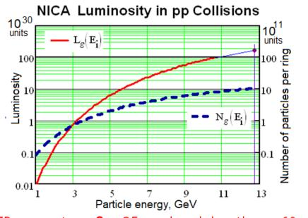
**□** IP parameters:  $\beta$  = 35 cm, bunch length  $\sigma$  = 60 cm **bunch number** – 22, collider perimeter **C** = 503 m
