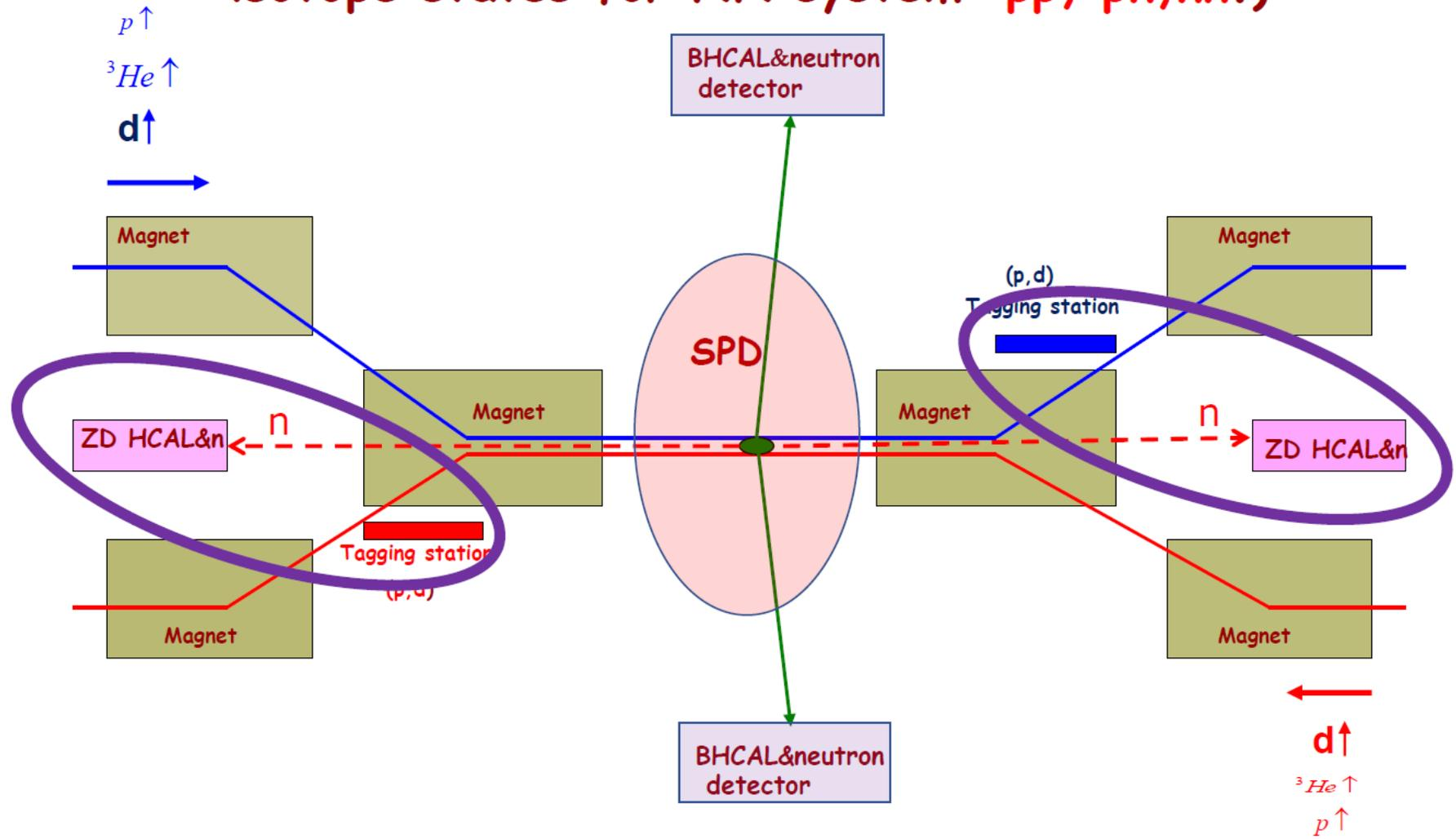
The tagging stations can be used as polarimeter!
